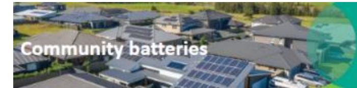
Community batteries provide a shared battery solution allowing residents to store excess power generated during the day by their rooftop solar cells for later use in the evening when demand on the electricity network is higher, or when the sun isn't shining.
